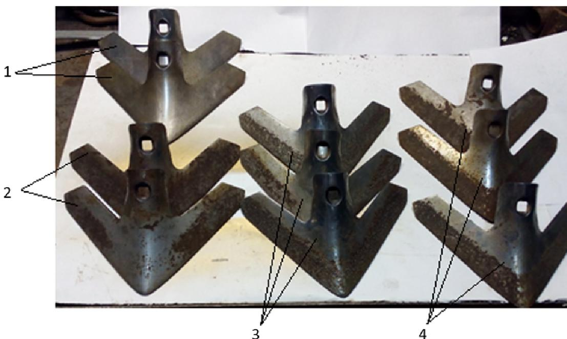
Fig. 3. Lancet paws after field work, reinforced with various electrodes:
